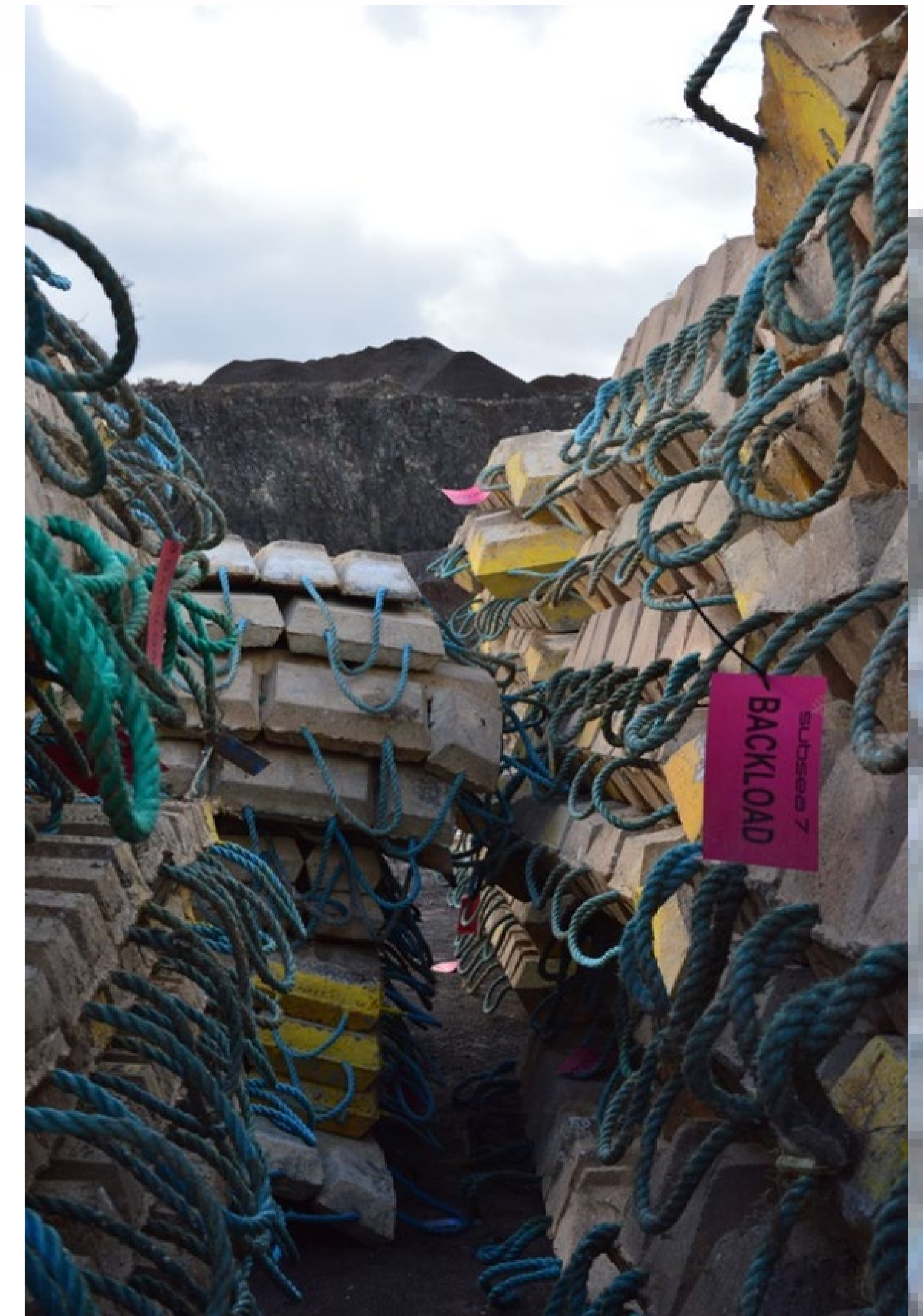
Concrete mattresses stored in quarry.
