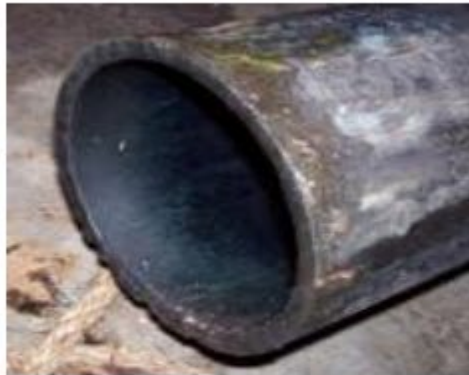
7" Inner casing recovered from concentric cut
