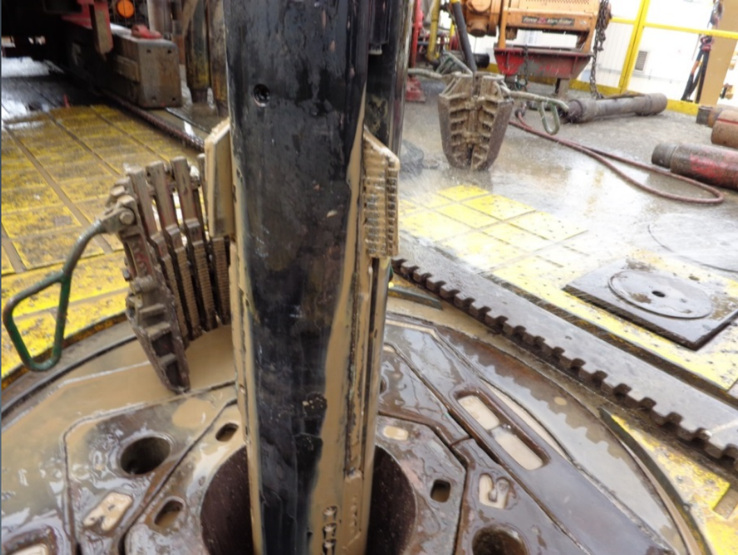
Endura® DSSM going through the Rotary Table during Testing
