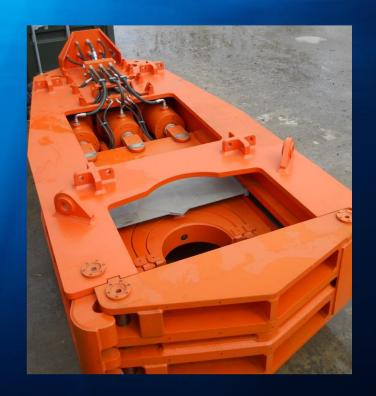
60" EVO<sup>™</sup> Super Shear – Currently Under Development Capable of shearing multistring reinforced pipe ≤60" Cutting force – 1555 Tons
