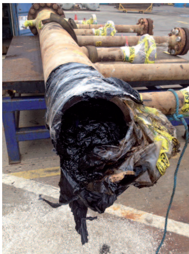
Figure 5: Receipt of pipelines at shore with considerable oil content. Source: Scotoil Services Limited (A Tradebe Company).
