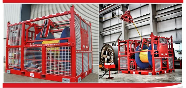
Brimmond group were approached by a multinational oil and gas service company to design and manufacture a bespoke downhole umbilical reeler for a project located in the Caspian Sea region. The details and specifications of the umbilical reeler and other equipment supplied were:
