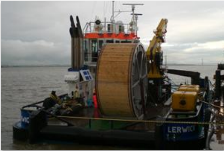
Multicat vessel with a cable drum
