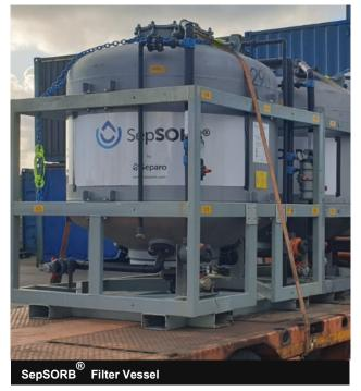
Hydrocarbon contaminated fluid was cleaned through the SepSORB® filter vessels and discharged overboard, well below the permitted 30ppm. The 2 x standby vessels were not required and were returned to the fleet for the next project.
