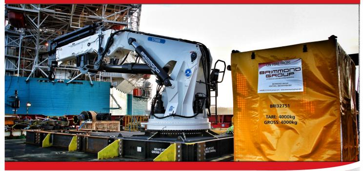
Brimmond Group were approached to supply an Effer 175000-6S marine knuckle boom crane to support a decommissioning project in the UK Continental Shelf. Brimmond's marine crane was utilised to manoeuvre and stack mattresses on deck which had been recovered from the seabed by the vessels main crane.
