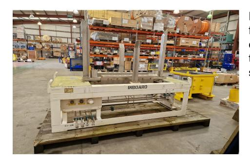
Here is Subsea Control Module Mounting Base that was unused from a Capital Project. J+S designed and remanufacturing it to our clients' requirements where, not only did this reduce the cost and the lead time for our client, but it also generated huge carbon savings.
